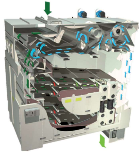
Figure 3 - Operation of a combi cleaner sieve.
